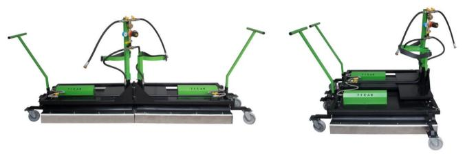
This equipment is intended for preparing the surface of the asphalt pavement for the restoration process in the case of small pothole repairs. Infrared heat warms up (dries) and effectively softens the road map for 5-7 minutes, while not impairing the properties of the asphalt (the bitumen does not burn out).
